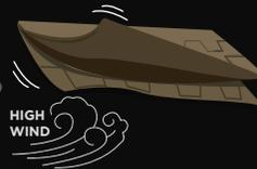
If not installed correctly, shingles could flap in the wind, stretching, creating loose nail holes, and eventually blowing off the roof.
