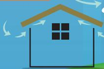
Less transfer of heat from the house, to the roof, means snow stays cold, blows off the roof, and does not easily turn into ice!
