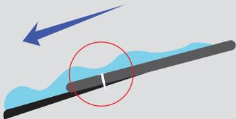
Allows for faster water flow, by reducing dips caused by the nail. This also makes it easy to hit **BOTH** layers every time.
